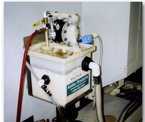
Model TKO-6 mounted to machine tool with CLO-1 magnetic frame.
